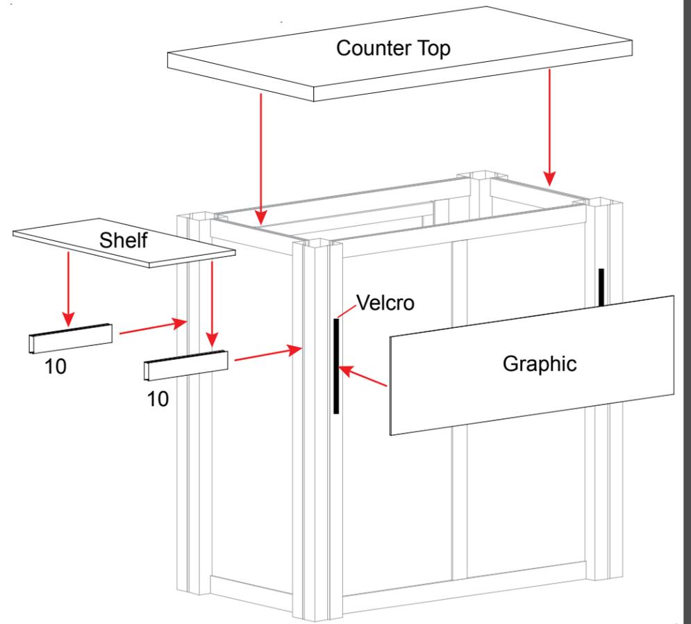
WHEN DISASSEMBLING ALUMINUM EXTRUSION, TIGHTEN ALL SETSCREWS AND LOCKS TO PREVENT LOSS DURING SHIPPING
